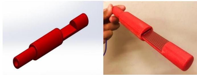
Figure 3 (a) Design of The Water Sensor Slot and (b) Actual Water Sensor Slot
